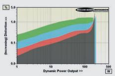
ABOVE: Dynamic power output versus distortion into 80hm (black trace), 40hm (red), 20hm (blue) and 10hm (green). Maximum current is 13.2A
